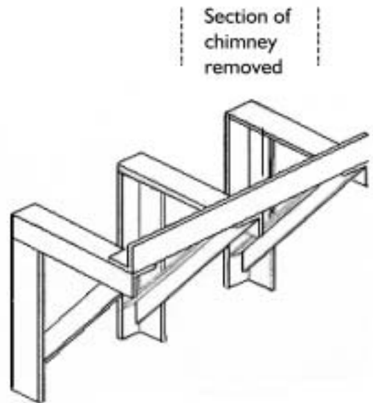
View of bracket in position
